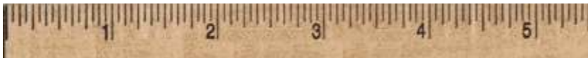
A ruler marked in 16ths. Every mark is 1/16th of an inch.
